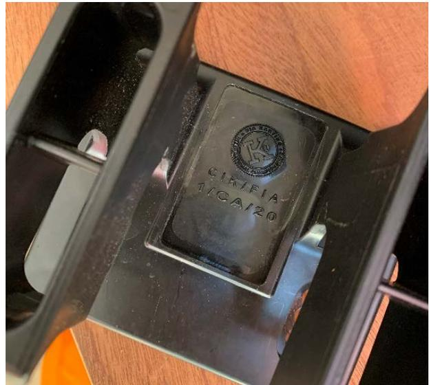
The photos depict the very early original CIK-FIA version of the dismountable block, which included a large cutaway so that when dismounted, the front fairing would drop significantly. This was quickly banned by CIK-FIA on safety grounds and the homologation of this version is no longer valid.
