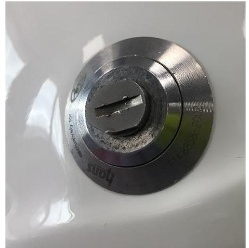
regulation K10.3.3(d). It was also noticed that the FHR posts were to the older FIA Standard 8858-2002, and are not compatible with a helmet to FIA Standard FIA 8859-2015, such as this one. The competitor admitted that he had swapped the FHR posts from his previous helmet without checking for compatibility. Remember the matrix showing the compatibility of FHR components and standards is available on motorsportuk.org in the Car Technical Resource Centre, which you can reach by [clicking here](#)
